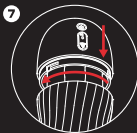
insert motors to the sleeve and close the housing
